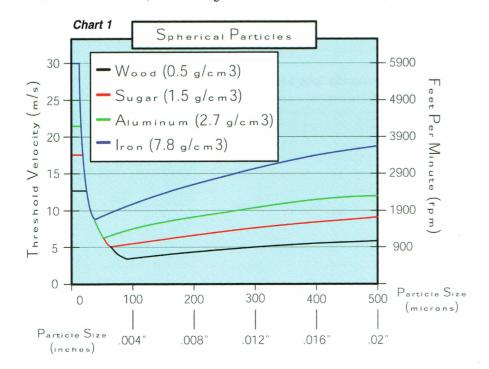
Towards Estimating Entrainment Fraction For Dust Layers (Authored by Erdem A. Ural). This shows the different velocity levels required to move four types of dust particles.
