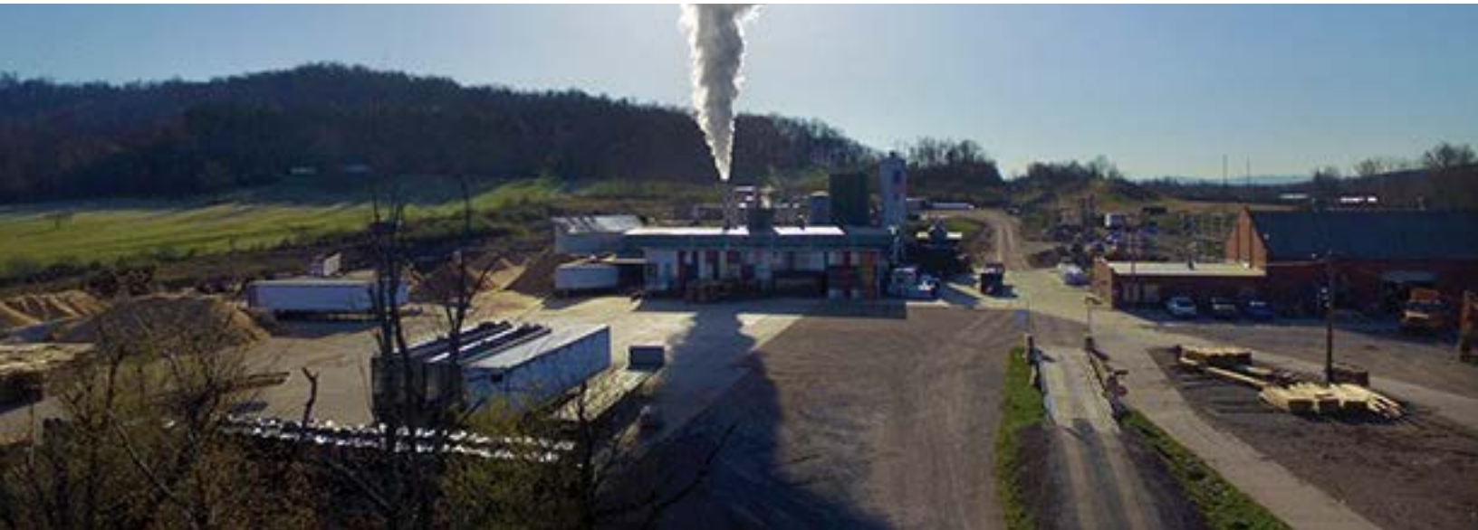
The Greene Team Pellet Fuel mill takes in at least five types of hardwood, including sawmill cutoffs, green sawdust, wood chips, dry sawdust and whole logs. PHOTO: GREENE TEAM PELLETT FUEL CO.
