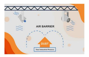
To minimize the dust build-up, they placed dust control fans strategically throughout their facility, as determined by SonicAire's specialized engineers. Now, when dust and fibers are released during processing, SonicAire fans create a barrier preventing dust from ever entering the ceiling area. Our BarrierAire technology forces dust to the ground, making clean-up an easy sweep-and-done operation that can be completed as a short daily task.
